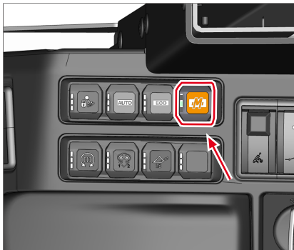
Fig. 89: Switch in the keypad for M-Drive
